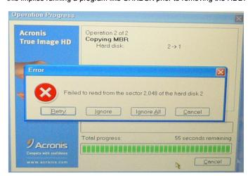
this implies running a program like CHKDSK prior to removing the HDD. This isn't a major issue, but running CHKDSK prior to cloning makes the cloning process easier.
